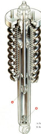
Coil-over shock absorbers are nitrogen gas filled and use a progressive-opening valve system.
