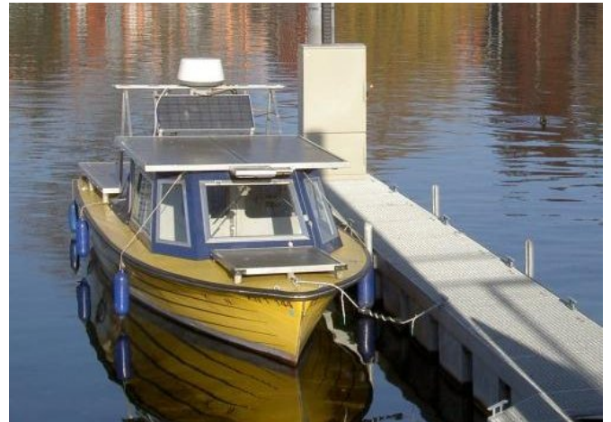
Fig. 1. The vessel Korona from the HTWG Konstanz equipped with the a Navico BR24 Radar Sensor.
